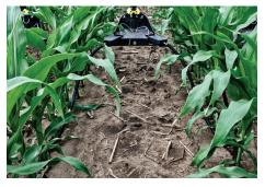
Four position adjustable arms allow for precision placement in 15-inch to 36-inch rows and variable rate nozzles are available for precise rate control.
