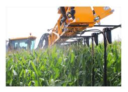
Breakaway mounting brackets and a flexible riser allow for easier navigation across hills and uneven terrain.
