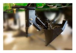
Breakaway risers provide protection on uneven terrain and variable rate nozzles are available for precise rate control.
