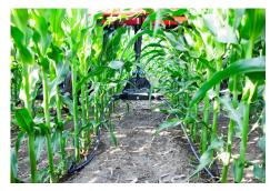
Adjustable riser length allows for mid to late season nitrogen application as late as V7 and four position adjustable arms allow for precision nitrogen placement in 15-36" rows.
