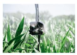
Easy add-on to 360 Y-DROP system – slides up and down the riser for vertical in-canopy positioning depending on crop growth stage.
