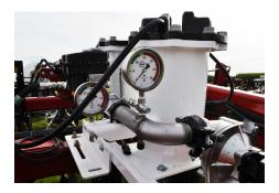
Centrifugal pump condenses NH3 into liquid for even application, regardless of rate and temperature.
