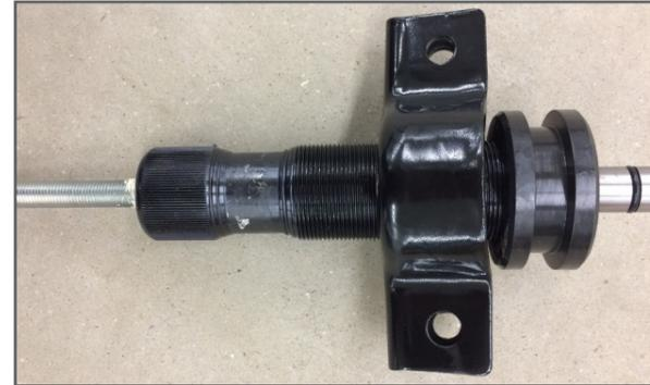
Thread the threaded bushing onto the hydraulic ram until it is in place with a few extra threads exposed on the side opposite of the threaded torque rod.
