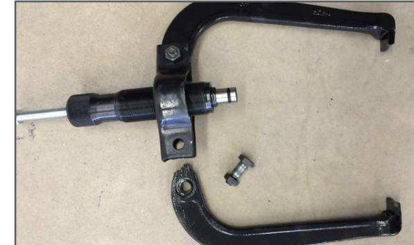
Attach the arm extension on one side with the bolt facing the appropriate way (reference Step 3). Attach the arm extension on the opposite side with the bolt facing the appropriate way (reference Step 3).
