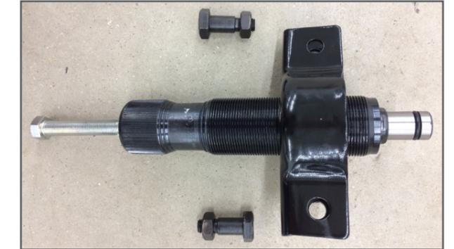
Before screwing the arms into the bracket and threaded bushing, notice the different sized holes on either side of the bracket. The head and nut of the bolt direction is opposite on each side, as shown. The smaller side hole is where you should secure the nut; the larger side hole is where the bolt head should sit.
