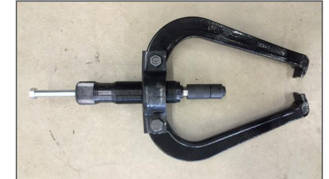
Install the extension shaft to protect the hydraulic ram, as shown. If you have factory/OEM stalk rolls for John Deere 40 and 90 series corn head models, use the John Deere 40-90 extension shaft.
